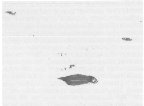
Fig. 6. Markedly elongated inclusions, in the lengthwise direction.
